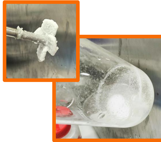
Crowning and deposition on reactor wall or propeller
